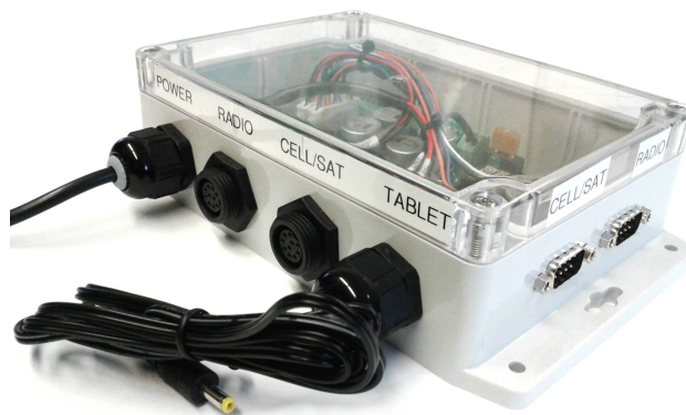
Figure 1.2: Serial Power Module showing labelled connections.
